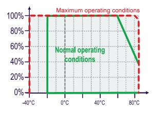
This chart shows the normal recommended operating range of the humidity sensor. Conditions outside the recommended range may temporarily offset the RH signal up to  $\pm 3$  %RH. After return to normal conditions it will slowly return towards calibration state by itself. See "Reconditioning Procedure" to accelerate this process. Prolonged exposure to extreme conditions may accelerate ageing.
